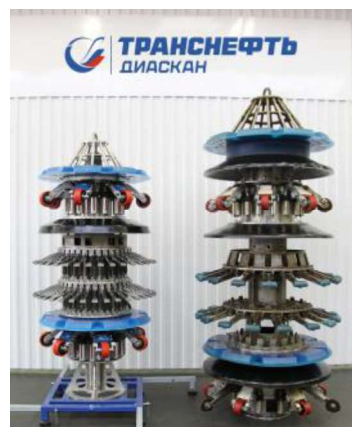
Transneft Diascan, JSC 's inline geometry inspection tool
