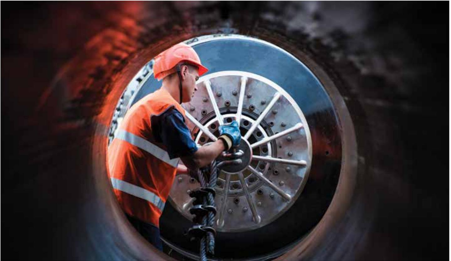
A combined magnetic and ultrasonic inspection tool is inserted into a pipeline.
